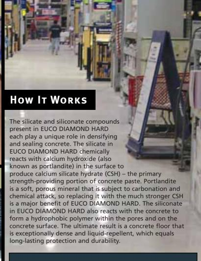
Silicate in EUCO DIAMOND HARD reacts with the calcium hydroxide present in concrete, producing a hard, crystalline gel called Calcium Silicate Hydrate (CSH). This gel fills the pores in the concrete surface, making it more dense and abrasion resistant.
